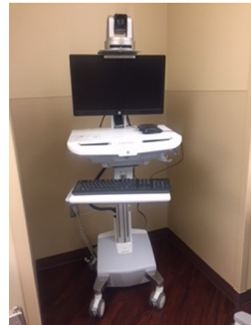
Image of the sepsis telehealth cart used for real clinical telehealth audiovisual connection and for the in situ simulation connection (our study) between the bedside care team and the eICU team.
