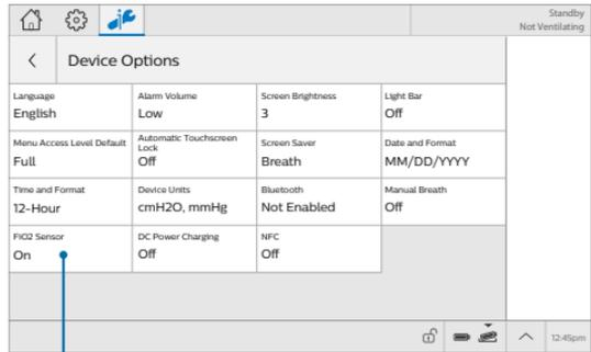
Under options, device options, tap the **FiO<sub>2</sub> Sensor** option and ensure the control is set to “On”
