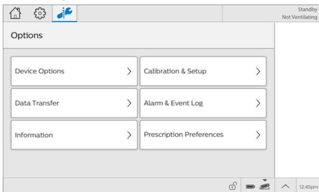
Within this window, change device options, run calibrations and tests, and view and work with data.
